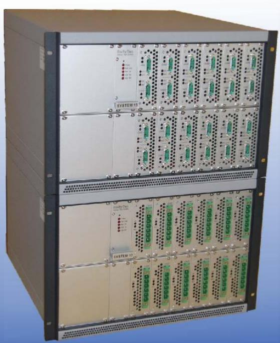
Cell Test and Formation System 25A or 50A output current with energy recovery
